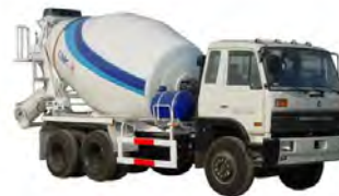
Cement Mixer Mix in Transit
